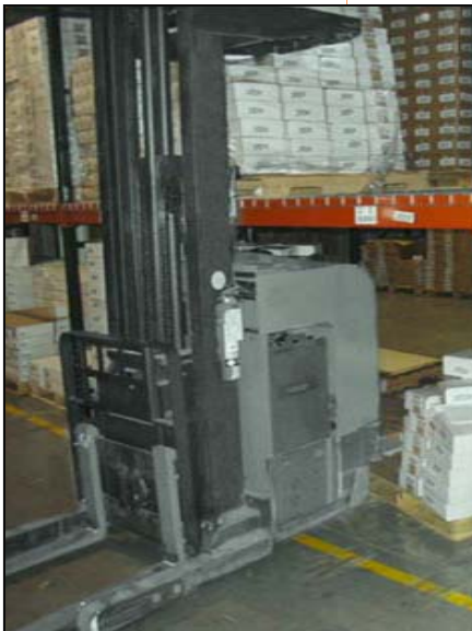
This photograph depicts a forklift under a storage rack after an under-ride accident. The crossbar is protruding above the operator's cab. Forklift manufacturers have various features available to assist in preventing such under-rides.
